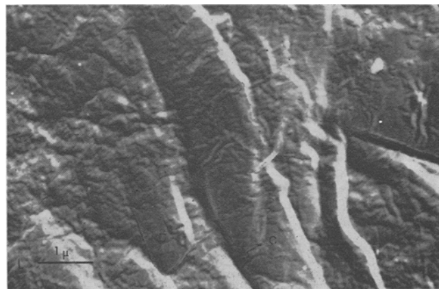
FIG. 2. A replica of a rapidly cooled lard. Crystals (C) can be seen beneath a masking layer of amorphous material. (Reduced approximately 45%)
