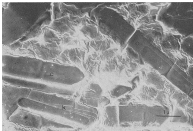
FIG. 10. A replica of a lard which had been treated with 35% aqueous Teepol, then slowly cooled. Crystals (C) composed of layers of crystallites (K) can be clearly seen. (Reduced approximately 45%)
